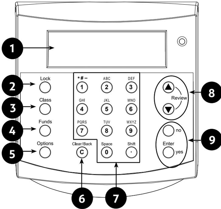
1. **LCD Display**—shows the current status of your DM50 Series meter and prompts you through all setup operations in a two-line LCD.
