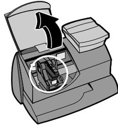
5. Press the top of the ink cartridge latch (on the green "unlock" icon).
