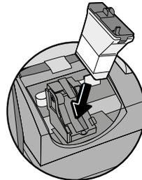
9. Press down on the ink cartridge latch firmly until it locks into place.
